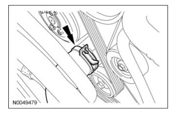
41. Connect the coolant hose to the thermostat housing.
