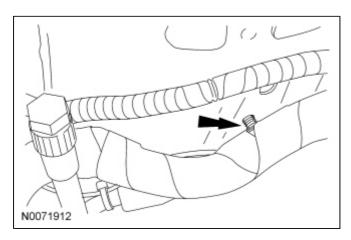
35. Attach the pin-type wire harness retainer to the cowl.
