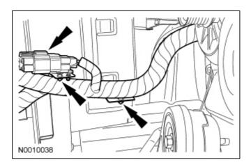
31. Connect the upper and lower PCM electrical connectors.
