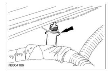
36. Connect the 2 heater hoses to the coolant tube assembly at the rear of the engine.
