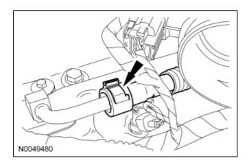
40. Connect the coolant hose to the coolant pump.
