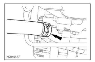
43. Connect the coolant hose from the Charge Air Cooler (CAC).
