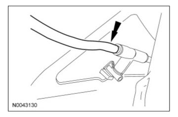
54. Install the hood insulation pin-type retainer and attach the 2 windshield washer hose retainers.
