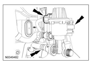
38. Connect the <u>EVAP</u> tube and brake booster vacuum supply tube to the Throttle Body (TB) spacer.
