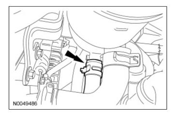
30. Connect the 16-pin electrical connector and attach the 2 wiring retainers
