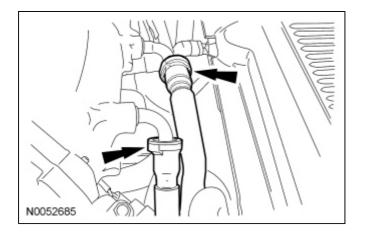
39. Connect the fuel supply tube. For additional information, refer to <u>Section 310-00</u>.
