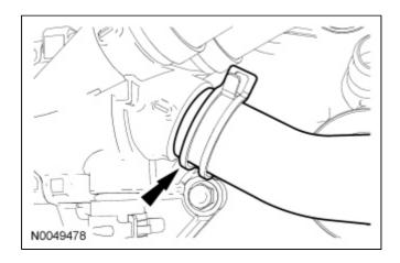
42. Connect the coolant hose to the coolant tube assembly (above the generator).
